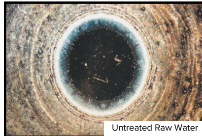
Photographs of Partially Evaporated Water Magnified to the 40th Power.
