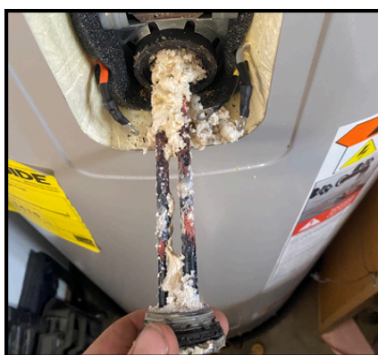
Severely Scaled Heating Element
