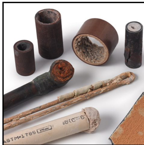
Scale buildup in various plumbing pipes (before Superior installed)
